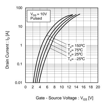
Fig.5 Typical Transfer Characteristics (I)
