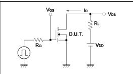
Fig.2-1 Gate Charge Measurement Circuit
