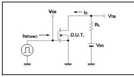
Fig.3-1 Switching Energy Measurement Circuit
