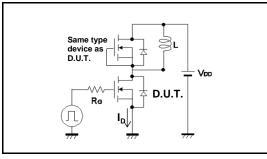
Fig.4-1 Reverse Recovery Time Measurement Circuit Fig.4-2 Reverse Recovery Waveform
