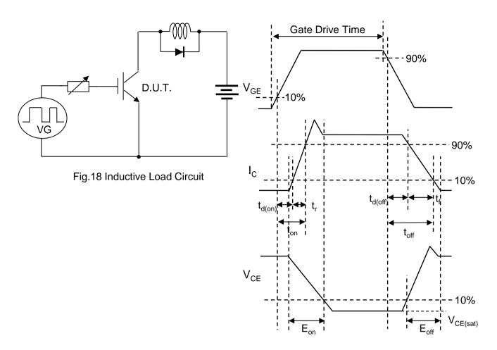
Fig.19 Inductive Load Waveform
