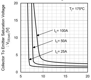
Gate To Emitter Voltage : V<sub>GE</sub> [V]
