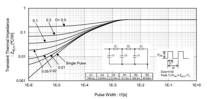
Fig.22 Typical Diode Transient Thermal Impedance
