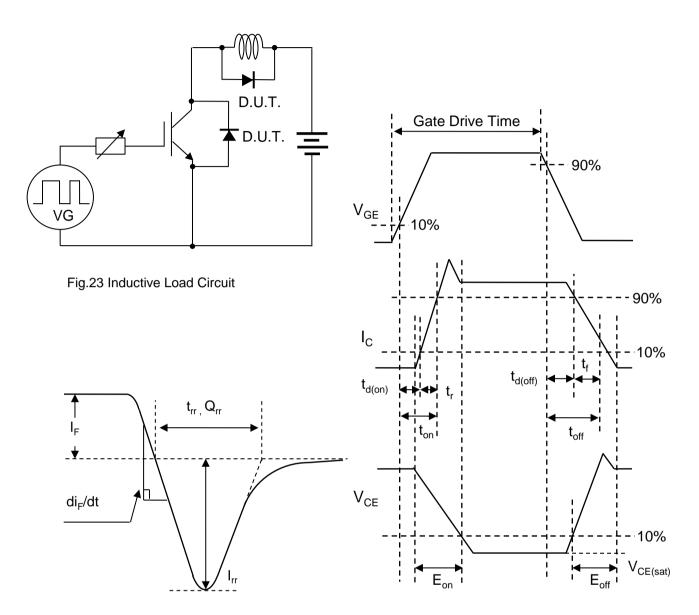
Fig.24 Diode Reverce Recovery Waveform
