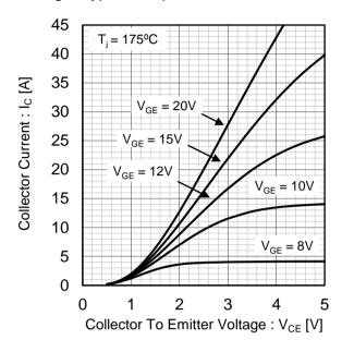
Fig.7 Typical Transfer Characteristics
