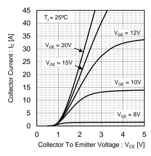
Fig.6 Typical Output Characteristics
