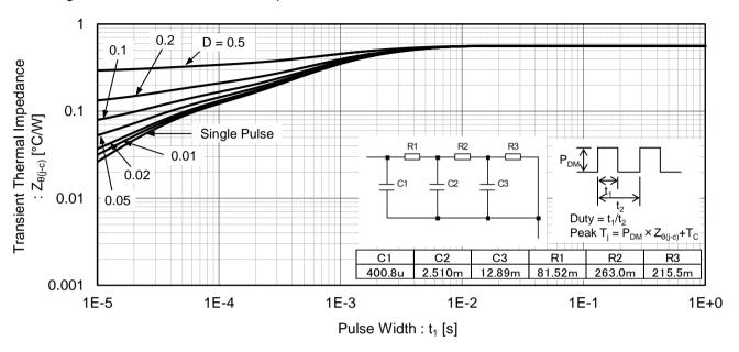
Fig.22 Diode Transient Thermal Impedance
