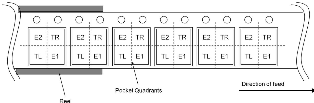
Fig.1 Quadrant Assignments for PIN 1 Orientation in Tape
