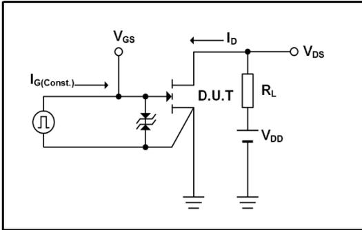
Fig.19 Switching Characteristics Measurement Circuit
