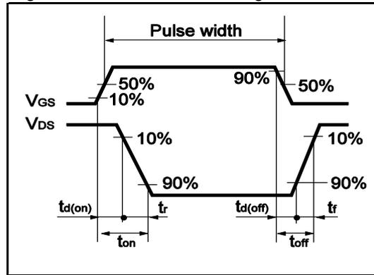
Fig.21 Waveforms for Switching Energy Loss
