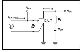
Fig.19 Switching Characteristics Measurement Circuit
