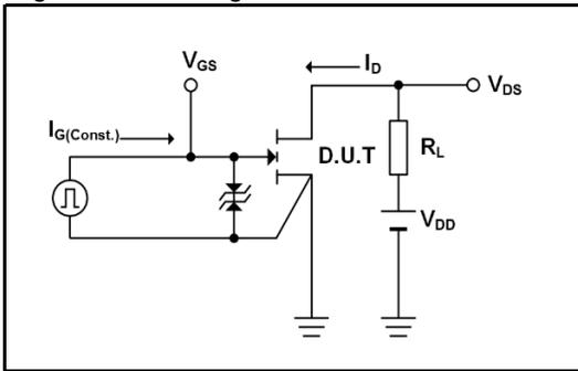
Fig.19 Switching Characteristics Measurement Circuit
