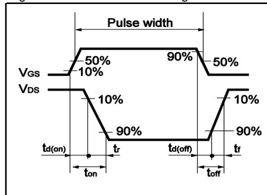
Fig.21 Waveforms for Switching Energy Loss
