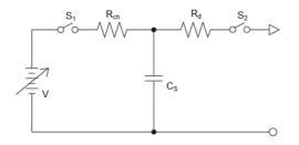
$\text{C}_{S}\text{:}150\text{pF} \;\; \text{R}_{d}\text{:}330\,\Omega$  simplified diagram in ESD machine
