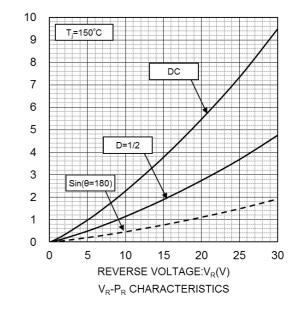
REVERSE POWER DISSIPATION:P<sub>R</sub>(W)
