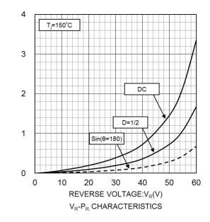
REVERSE POWER DISSIPATION:P<sub>R</sub>(W)
