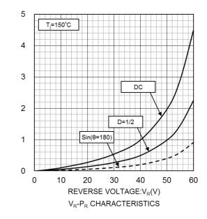
REVERSE POWER DISSIPATION:P<sub>R</sub>(W)
