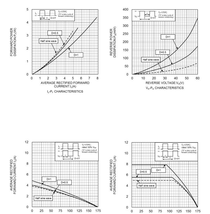
CASE TEMPERATURE: $T_{C}(^{\circ}C)$ DERATING CURVE(I<sub>0</sub>- $T_{C}$ )
