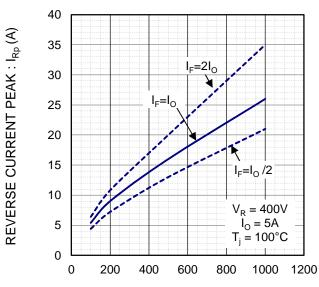
RATE OF CHANGE OF CURRENT :  $-di/dt(A/\mu s)$   $di/dt-I_{Rp}$  CHARACTERISTICS
