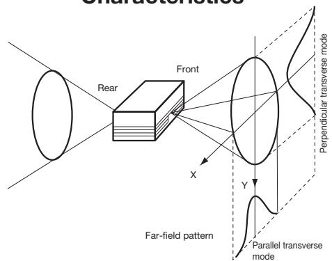
**Fig.4 Radiation Characteristics**
