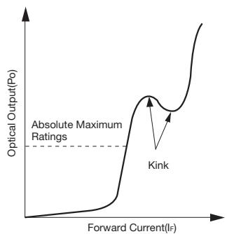
**Fig.2 Optical Output vs. Forward Current**
