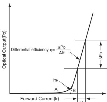
**Fig.3 Radiation Characteristics**
