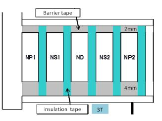
Core: JFE MB3 EER-28.5A or compatible Bobbin: JFE BER28.5SP12 Vertical/Terminal Pins 6-6(12pins) or compatible AL-Value: 149.4 nH/N<sup>2</sup>
