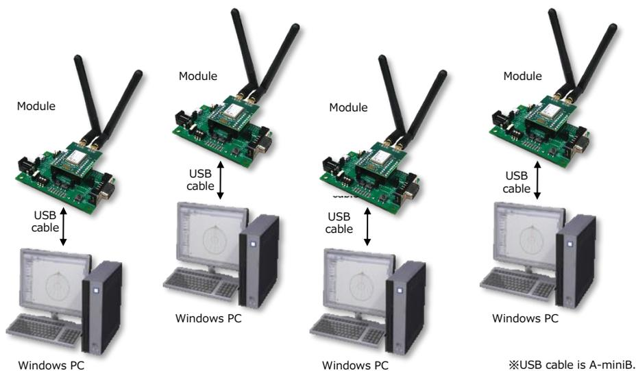
**Figure 1. System Configuration Example of 4 PCs**
