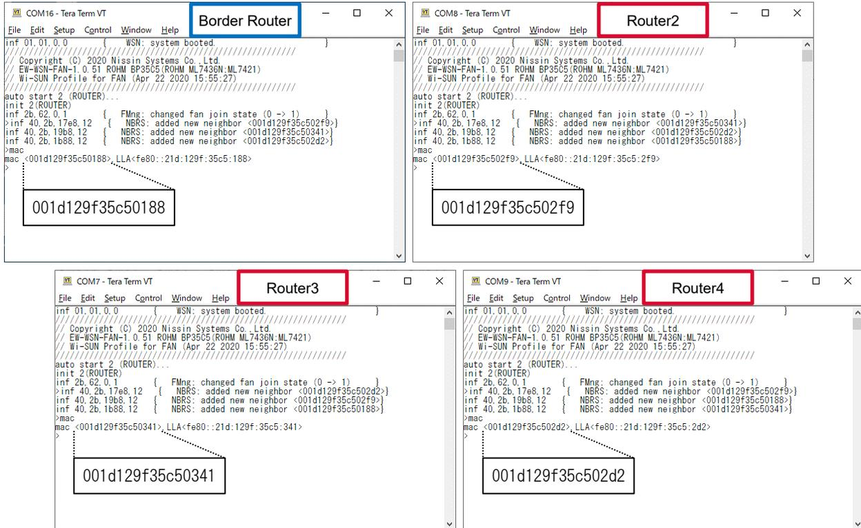
Figure 7. Checking of MAC Address by Command
