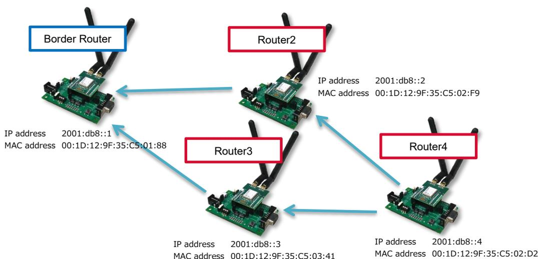
Figure 4. Mesh Networking Configuration Diagram
