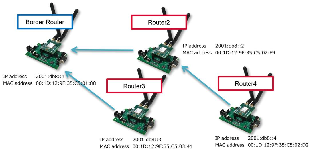
**Figure 13. Mesh Networking Connection**
