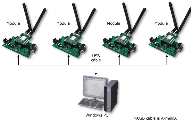
**Figure 2. System Configuration Example of 1 PC**
