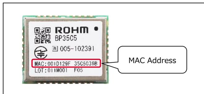
Figure 8. Checking of MAC Address by Label
