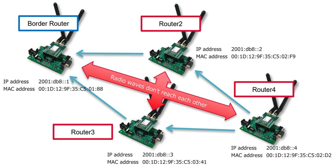
**Figure 9. Mesh Networking of Sample Script**
