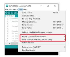
Figure 3. Board and COM Port setting
