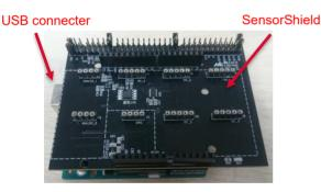
Figure 1. Connection between the Arduino and the SensorShield
