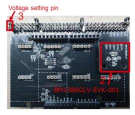
Figure 2. Connection between BM1386GLV-EVK-001 and the SensorShield
