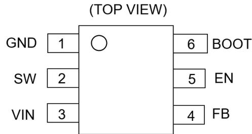
Figure 3. Pin Configuration
