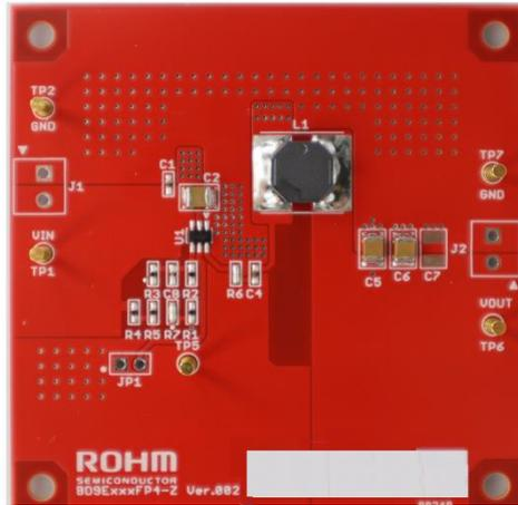
Figure 1. Evaluation Board Top View
