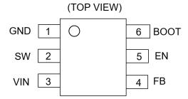
Figure 3. Pin Configuration
