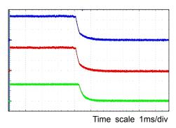
Figure 16. Power-down EN =  $V_{IN}$  $V_{IN}$  = 12V,  $V_{O}$  = 3.3V,  $I_{O}$  = 0A
