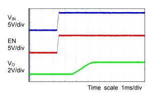
Figure 15. Start-up EN =  $V_{IN}$  $V_{IN}$  = 12V,  $V_{O}$  = 3.3V,  $I_{O}$  = 0A
