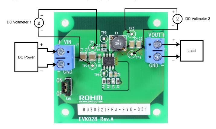
Figure 1. Connection Diagram
