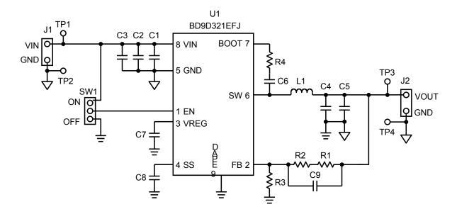
Figure 2. BD9D321EFJ-EVK-001 Circuit Diagram
