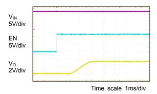
Figure 17. Start-up by EN  $V_{IN}$  = 12V,  $V_O$  = 3.3V,  $I_O$  = 0A
