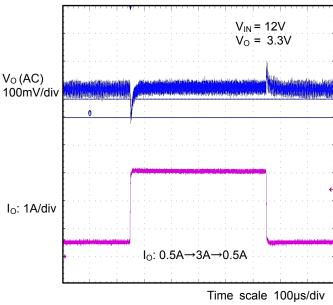
Figure 12. Load Transient Characteristics
