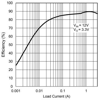
Figure 9. Efficiency vs Load Current
