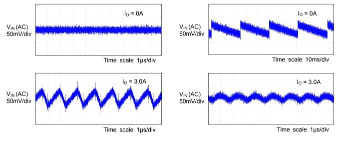
Figure 13. Input Voltage Ripple Wave  $V_{IN}$  = 12V,  $V_{O}$  = 3.3V
