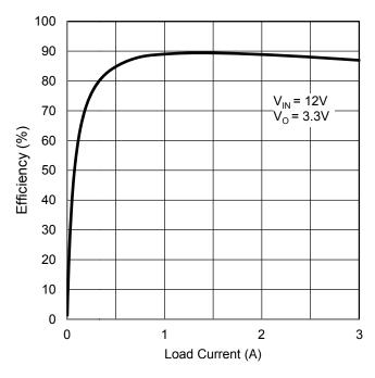
Figure 9. Efficiency vs Load Current
