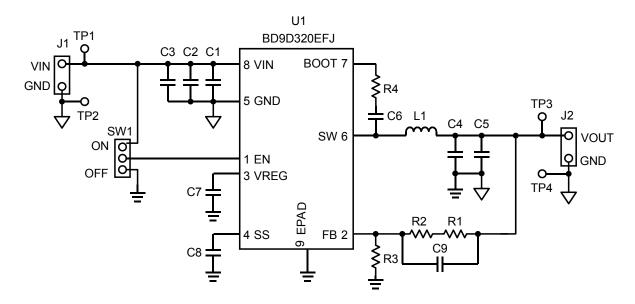
Figure 2. BD9D320EFJ-EVK-001 Circuit Diagram
