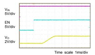
Figure 17. Start-up by EN  $V_{IN}$  = 12V,  $V_O$  = 3.3V,  $I_O$  = 0A
