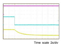
Figure 18. Power-down by EN  $V_{IN}$  = 12V,  $V_O$  = 3.3V,  $I_O$  = 0A
