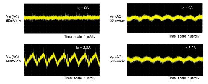
Figure 13. Input Voltage Ripple Wave  $V_{IN}$  = 12V,  $V_{O}$  = 3.3V
