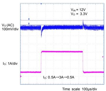
Figure 12. Load Transient Characteristics
