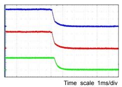
Figure 16. Power-down EN =  $V_{IN}$  $V_{IN}$  = 12V,  $V_{O}$  = 3.3V,  $I_{O}$  = 0A
