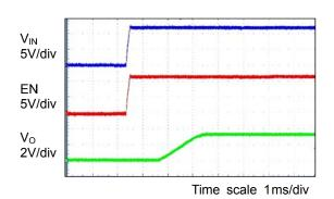
Figure 15. Start-up EN =  $V_{IN}$  $V_{IN}$  = 12V,  $V_{O}$  = 3.3V,  $I_{O}$  = 0A
