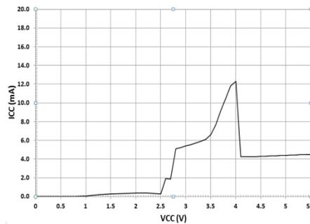
Fig 5: Circuit Current vs. Power Supply Voltage (Temp=25°C, FREQ=L, MODE=L)
