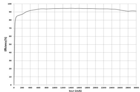
Fig 6: Electric Power Conversion Rate ( $V_{OUT}=3.3V$ , FREQ=L, MODE=L)
