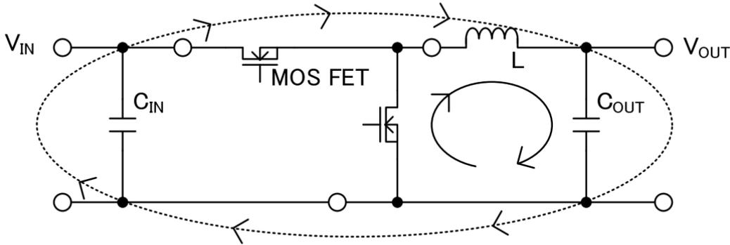
**Fig 32: Current Loops of Buck Regulator System**
