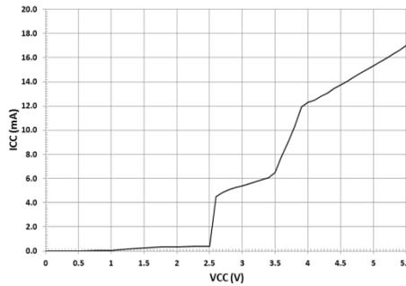
Fig 12: Circuit Current vs. Power Supply Voltage (Temp=25°C, FREQ=L, MODE=H)
