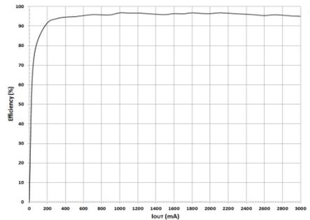
Fig 27: Electric Power Conversion Rate ( $V_{OUT}=3.3V$ , FREQ=H, MODE=H)
