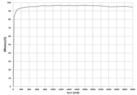
Fig 20: Electric Power Conversion Rate ( $V_{OUT}=3.3V$ , FREQ=H, MODE=L)
