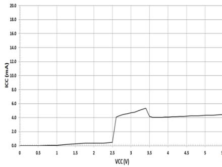
Fig 19: Circuit Current vs. Power Supply Voltage (Temp=25°C, FREQ=H, MODE=L)
