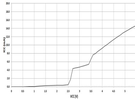
Fig 26: Circuit Current vs. Power Supply Voltage (Temp=25°C, FREQ=H, MODE=H)
