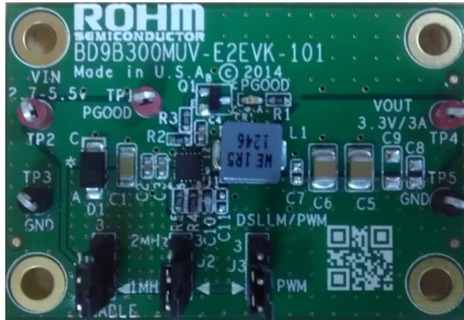
Fig 1: Evaluation Board for the BD9B300MUV
