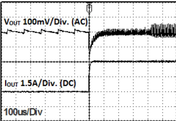
Fig 21: Load Response Characteristics ( $V_{IN}=5V$ ,  $V_{OUT}=3.3V$ ,  $I_{OUT}=0 \rightarrow 3A$ , FREQ=H, MODE=L)
