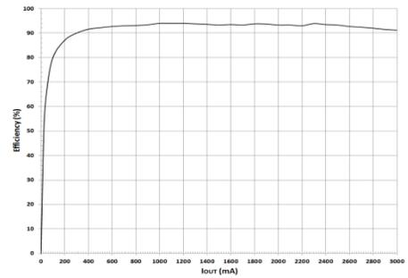
Fig 13: Electric Power Conversion Rate ( $V_{OUT}=3.3V$ , FREQ=L, MODE=H)
