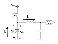
Figure 1-a. Asynchronous Buck Converter
