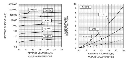
Figure 5. Rohm Schottky Barrier Diode RSX301LAW30 Characteristic Curve for Reverse Loss
