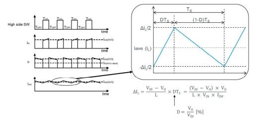
Figure 3. Illustration of Ripple Current
