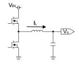
Figure 1-b. Synchronous Buck Converter
