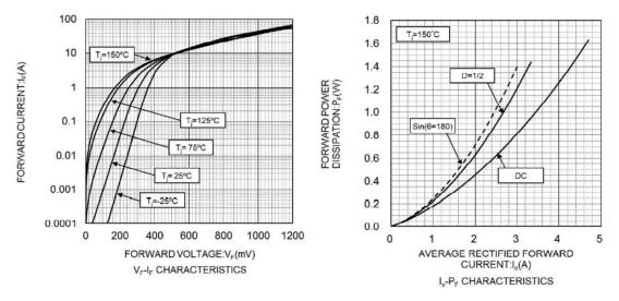
Figure 4. Rohm Schottky Barrier Diode RSX301LAW30 Characteristic Curve for Forward Loss
