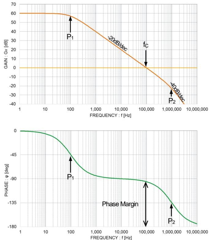
Figure 1. Bode plot for NPN-type LDO
