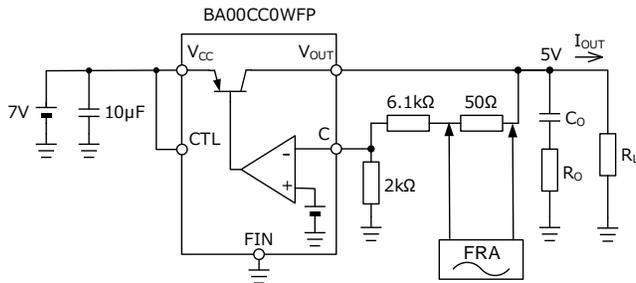
Figure 9. Evaluation circuit for stable operation
