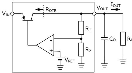
Figure 2. Circuit diagram of BAxxCC0 series LDO
