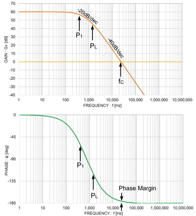
Figure 3. Bode plot for PNP-type LDO Without phase compensation
