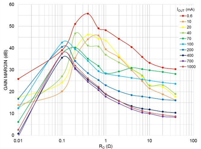
Figure 11. Gain margin vs.  $R_o$
