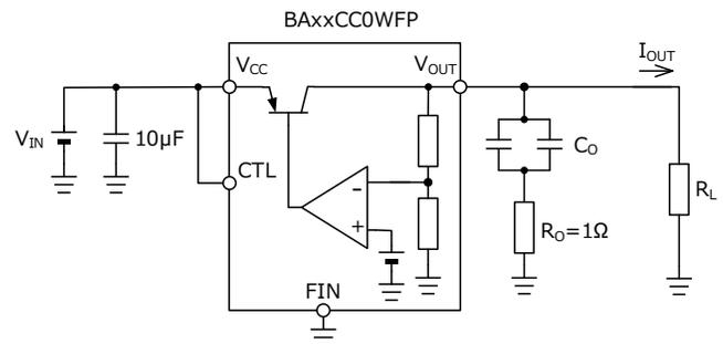
Figure 15. Circuit using an output ceramic capacitor
