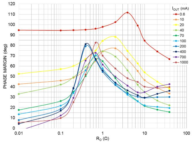
Figure 10. Phase margin vs.  $R_o$
