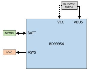
Figure 23. Set Up for Battery Charging
