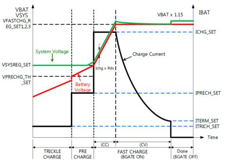
Figure 22. Battery Charging Profile
