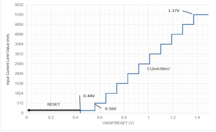
Figure 31. IADP Pin Input Current Limit Settings
