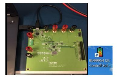
Figure 9. USB-I2C Communication Set Up and Desktop Shortcut
