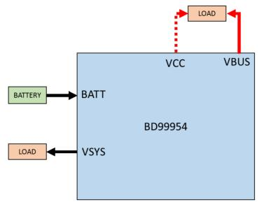
Figure 29. Set Up for Reverse Buck-Boost Operation
