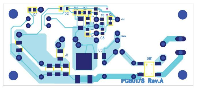
Figure 6. Bottom Layout (Bottom view)
