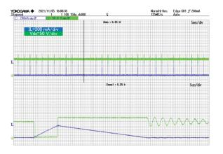
Figure 11 Vds and IL VIN = 90 Vac, IOUT = 0 A
