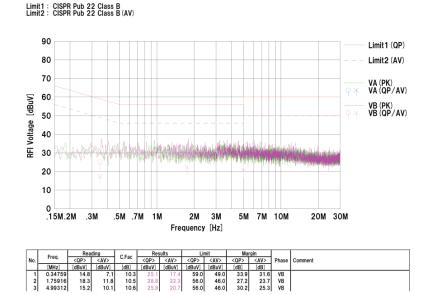
Figure 28. Conduction Noise VIN = 90 Vac
