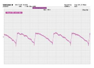
Figure 26. Vout Ripple Voltage (5MHz filter) VIN = 264 Vac, IOUT = 0.417 A
