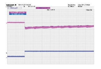
Figure 21. lout and Vout (5 MHz Filter) VIN = 90 Vac, IOUT = 0.05 A to 0.417 A
