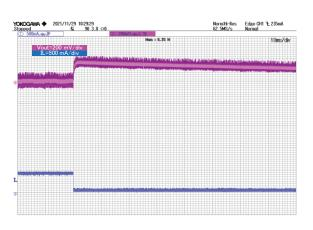
Figure 24. lout and Vout (5 MHz Filter) VIN = 264 Vac, IOUT = 0.417 A to 0.05 A
