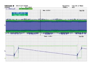
Figure 16. Vds and IL VIN = 264 Vac, IOUT = 0.417 A
