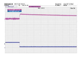
Figure 23. lout and Vout (5 MHz Filter) VIN = 90 Vac, IOUT = 0.417 A to 0.05 A
