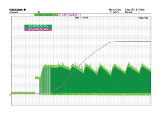
Figure 19. Vds and Vout VIN = 90 Vac, IOUT = 0.417 A
