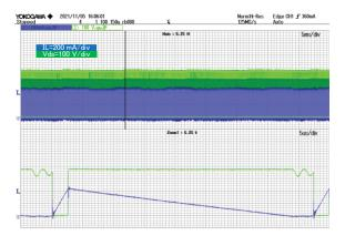
Figure 14. Vds and IL VIN = 264 Vac, IOUT = 0.2 A
