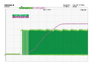
Figure 20. Vds and Vout VIN = 264 Vac, IOUT = 0.417 A
