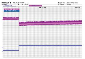
Figure 22. lout and Vout (5 MHz Filter) VIN = 264 Vac, IOUT = 0.05 A to 0.417 A
