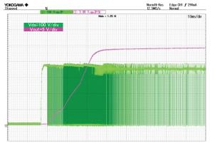
Figure 18. Vds and Vout VIN = 264 Vac, IOUT = 0 A
