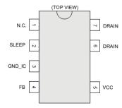
Figure 7. Pin Configuration
