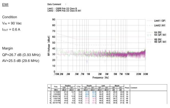
Figure 28. Conduction Noise VIN = 90 Vac
