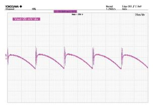
Figure 25. Vout Ripple Voltage (5 MHz Filter) VIN = 90 Vac, IOUT = 0.6 A
