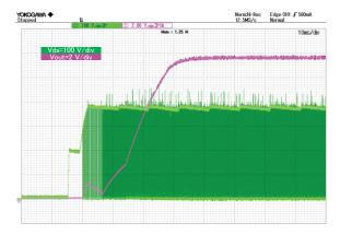
Figure 20. Vds and Vout VIN = 264 Vac, IOUT = 0.6 A
