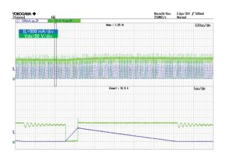
Figure 13. Vds and IL VIN = 90 Vac, IOUT = 0.3 A
