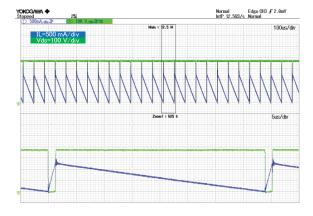
Figure 16. Vds and IL VIN = 264 Vac, IOUT = 0.6 A
