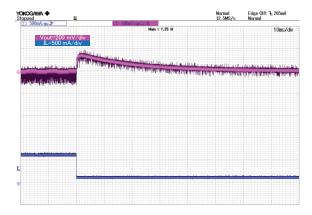
Figure 24. lout and Vout VIN = 264 Vac, IOUT = 0.6 A to 0.1 A
