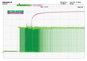
Figure 17. Vds and Vout VIN = 90 Vac, IOUT = 0 A
