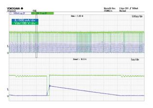
Figure 14. Vds and IL VIN = 264 Vac, IOUT = 0.3 A
