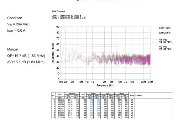
Figure 29. Conduction Noise VIN = 264 Vac
