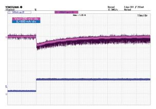
Figure 21. lout and Vout VIN = 90 Vac, IOUT = 0.1 A to 0.6 A
