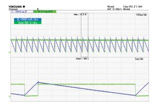
Figure 15. Vds and IL VIN = 90 Vac, IOUT = 0.6 A
