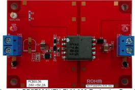
Figure 1. BD7F200HFN-EVK-002 Evaluation Board Top View
