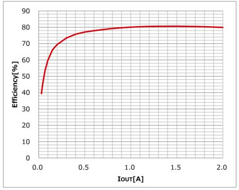
Figure 11. Efficiency vs Load Current
