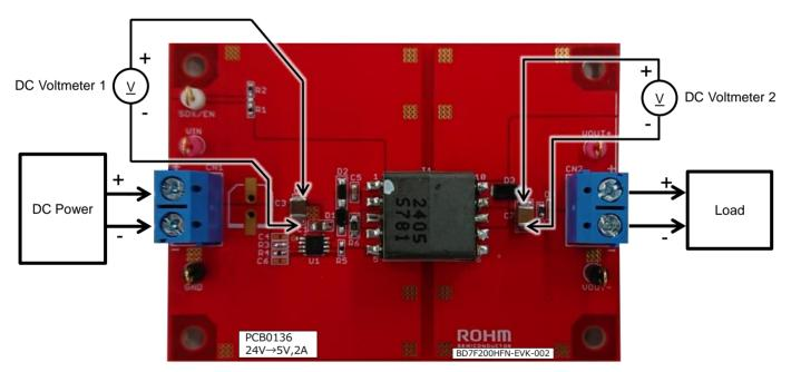
Figure 3. Connection Diagram
