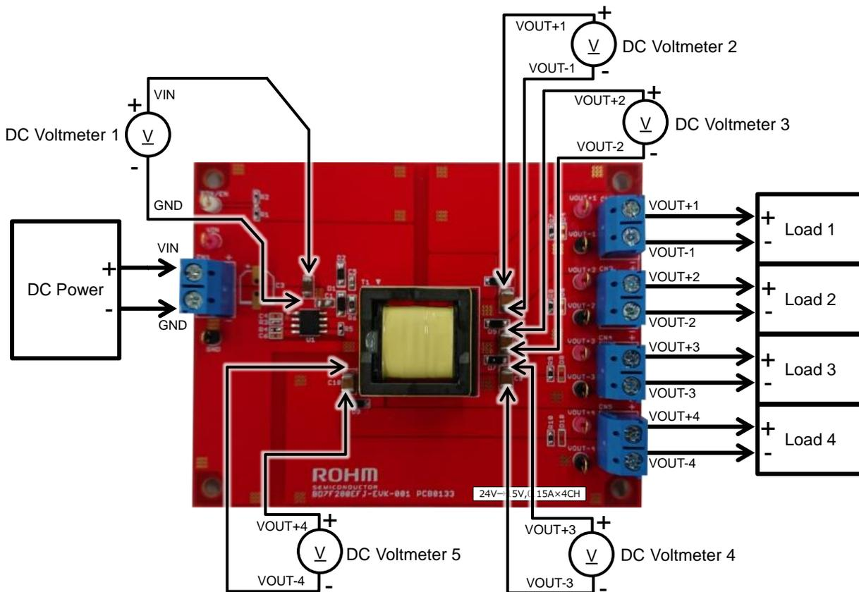
Figure 3. Connection Diagram
