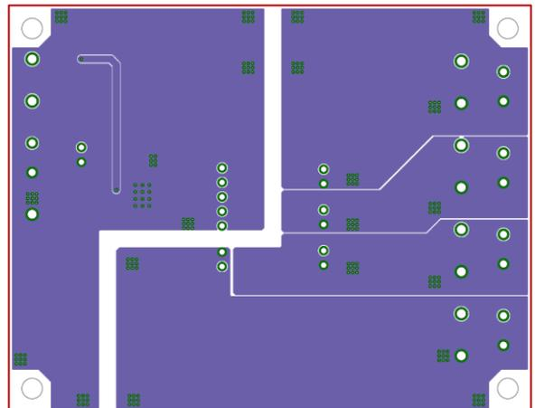
Figure 10. Bottom Side Layer Layout
