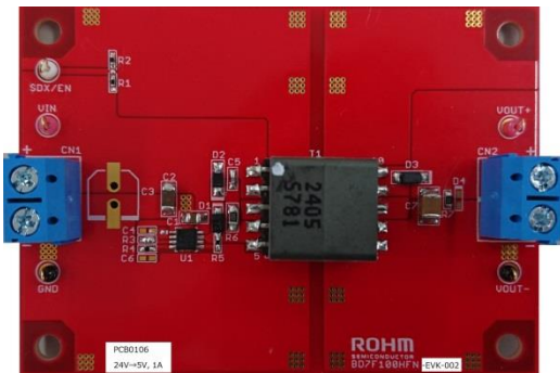
Figure 1. BD7F100HFN-EVK-002 Evaluation Board
