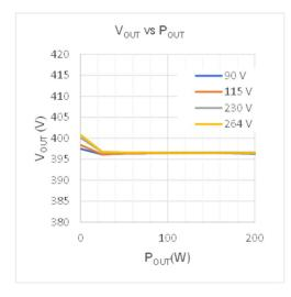
Figure 7. Load Regulation (V\_oUT vs P\_OUT)
