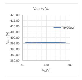
Figure 8. Line Regulation ( $V_{OUT}$  vs  $V_{IN}$ )
