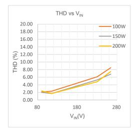
Figure 9. Tatal Harmonic Distortion (THD vs  $V_{IN}$ )
