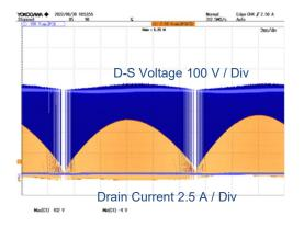
Figure 16. VDS,ID VIN = 90 Vac IOUT = 0.5 A
