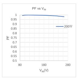
Figure 10. Power Factor (PF vs VIN)
