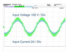
Figure 14. Input Current  $V_{IN}$  = 115  $V_{ac}$ ,  $I_{OUT}$  = 0.5 A
