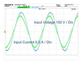
Figure 15. Input Current  $V_{IN}$  = 230  $V_{ac}$ ,  $I_{OUT}$ =0.5 A
