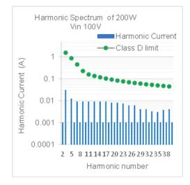
Figure 12. Harmonic Current VIN = 100 Vac
