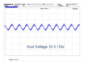
Figure 23. Output ripple VIN = 90 Vac
