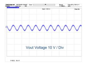
Figure 24. Output ripple VIN = 264 Vac
