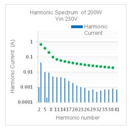
Figure 13. Harmonic Current VIN = 230 Vac
