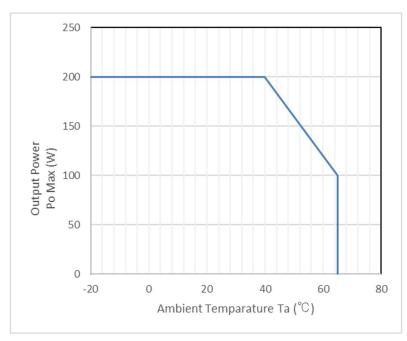
Figure 2. Temperature derating curve
