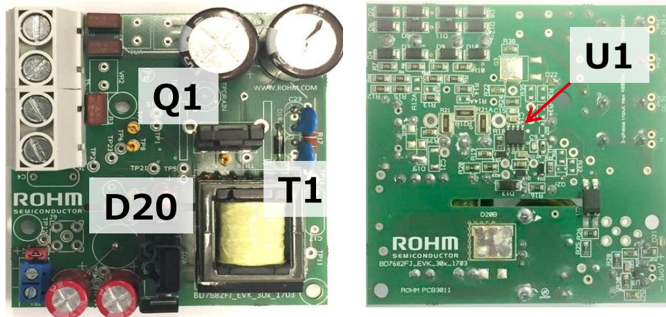
Figure 6 – Top side (left) and bottom side (right) of the AUX board.
