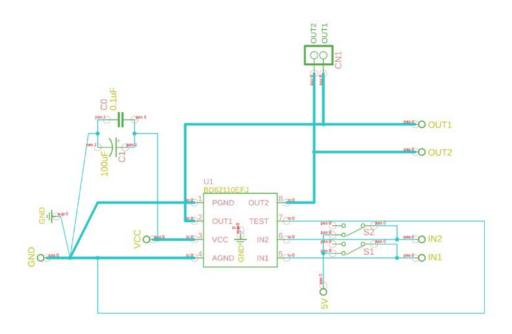
Figure 8. Evaluation board schematic
