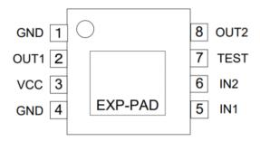
Figure 7. Pin configuration
