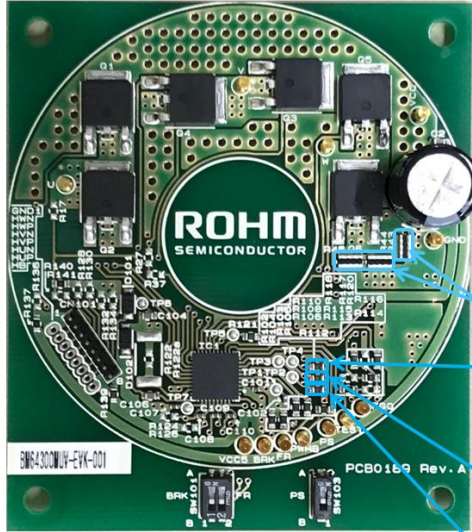
&lt;Front, pre-driver and MOS (TO252) mounted surface&gt;
