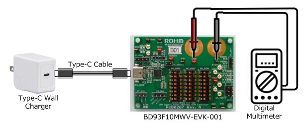
Note that changing the configuration via each DIP switch requires the power cycle to be updated, so please disconnect the source device from EVK by removing a cable.
