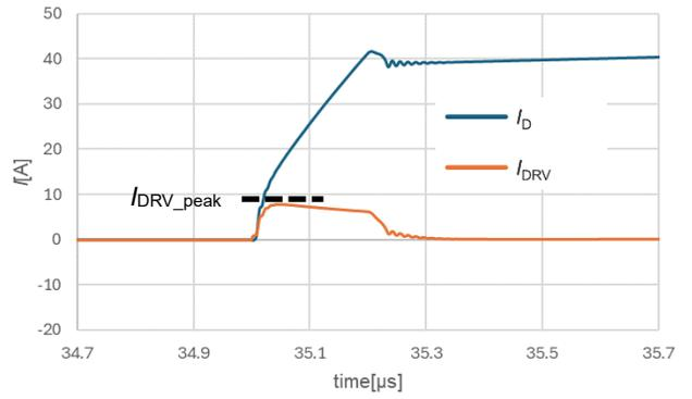
(z)  $L_{SOURCE} = 30nH, R_G = 2.2ohm, R_{DSS} = 1ohm$
